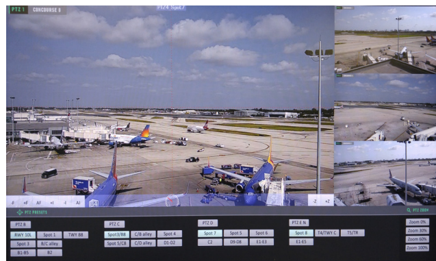
FLL: Virtual Ramp Control System
